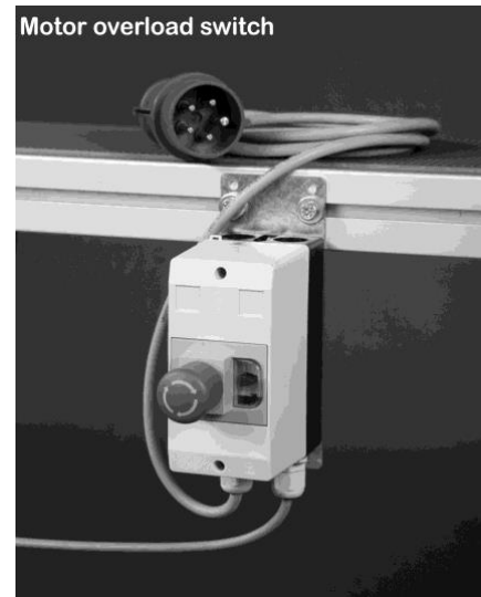
Figure 3-13: Motor overload switch
