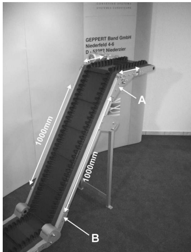
Figure 4-12: Axial distances on Z-shaped belt conveyor
