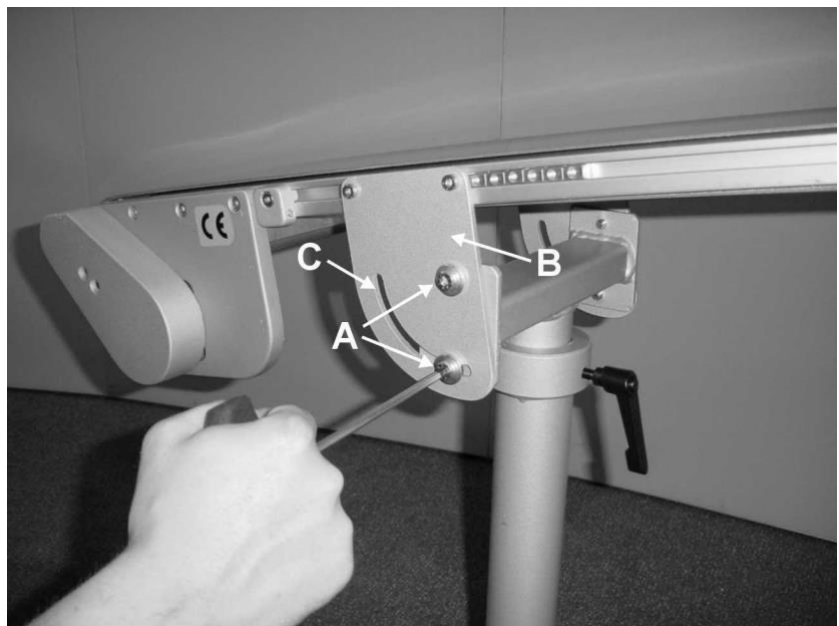
Figure 4-21: Single-legged steel support with aluminium base plate, inclination adjustment
