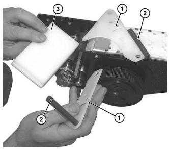
14. Loosen two set screws (Figure 166, item 1) on two bearings (Figure 166, item 2).
