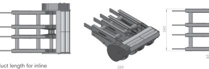
Minimum product length for inline transfer = 100 mm Transfer extends past conveyor
