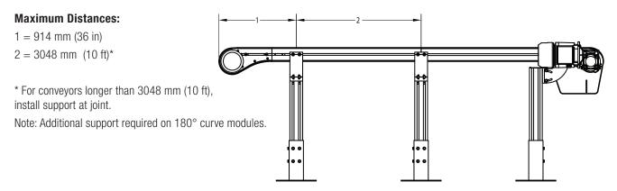
Support must be provided directly at drive end. See accessories for Direct Mount and Suspended Mount support options.
