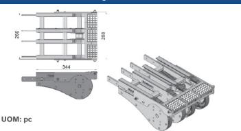
End transfer bridge c/w roller for FVIE-A260, FVDD-A260-XDY and FVDD-A260GP-XDY
