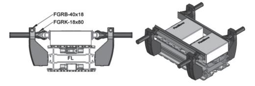
Width & Height Adjustable Guide Rail Assembly
