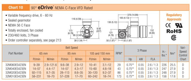
\* = At 60 Hz \*\* = Motor is de-rated to 0.5 Hp (2.2 / 1.1 amp) for full torque throughout the speed range.
