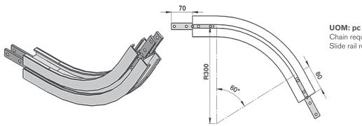
Chain required 2-way: 0.9 meter Slide rail required 2-way: 1.9 meter
