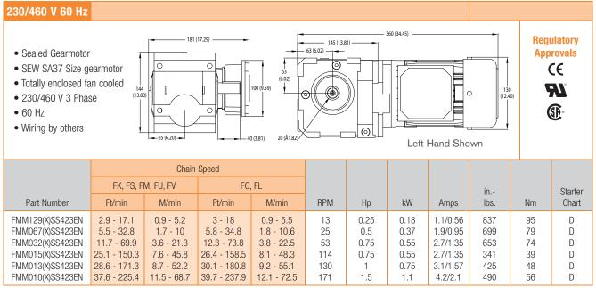
Where (X) is L or R for Right Hand or Left Hand Gearmotor matching RH or LH Drive
