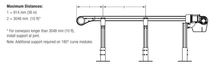
Support must be provided directly at drive end. See accessories for Direct Mount and Suspended Mount support options.
