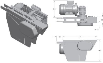
Minimum product length for inline transfer = 100 mm Provides extended transfer nose for interfacing with large rollers.
