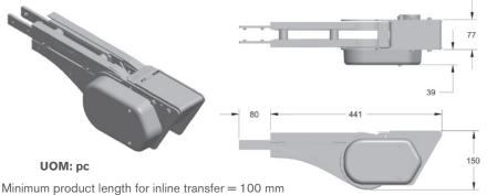
Provides extended transfer nose for interfacing with large rollers.
