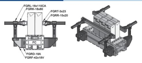
Width & Height Adjustable Guide Rail Assembly
