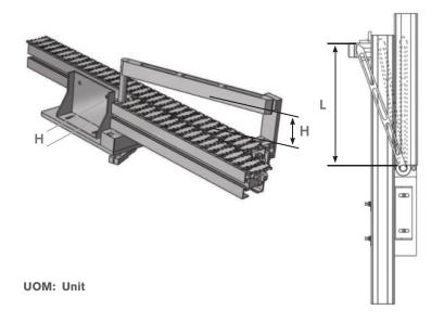
**Application:** Pneumatic-controlled automatic diversion of products from one track to another
