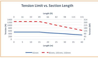
To calculate the Nominal Maximum Load: *Note: This does not include conveyor configuration. Please confirm load with Dorner online DTools configurator.*
