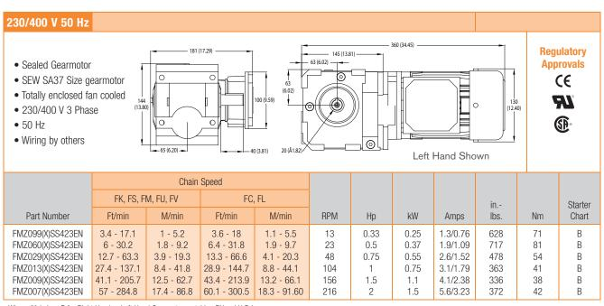
Where (X) is L or R for Right Hand or Left Hand Gearmotor matching RH or LH Drive
