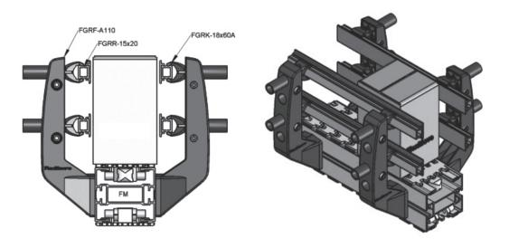
Width Adjustment Guide Rail Assembly
