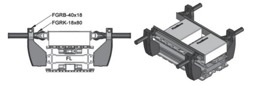
Width & Height Adjustable Guide Rail Assembly
