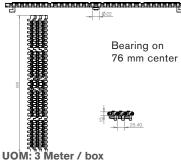
Application: Suitable for horizontal and slope >5 Degree but </= 25 Degree transport of products without accumulation
