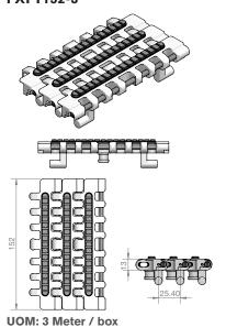
Application: Suitable for horizontal and slope >5 Degree but </= 25 Degree transport of products without accumulation
