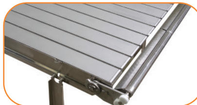
OPTIONAL: Stainless Steel or UHMW Bedplates
