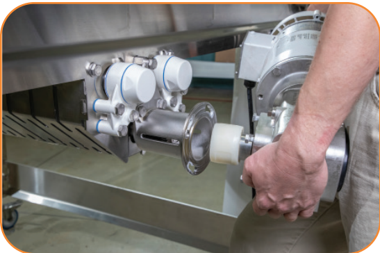
QUICK REMOVAL SIDE MOUNT GEARMOTOR TO REDUCE SANITATION TIME
