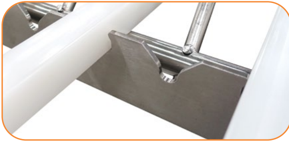
All surfaces on internal frame components are polished to 32 microinch, except belted product.
