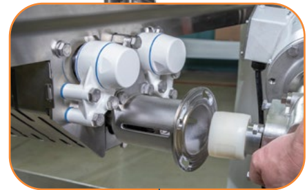
QUICK REMOVAL SIDE MOUNT GEARMOTOR TO REDUCE SANITATION TIME
