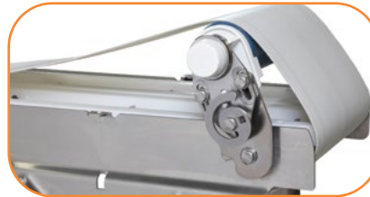
STANDARD FEATURE: Tip-Up Tail**
