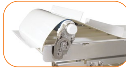
STANDARD FEATURE: Tip-Up Tail**
