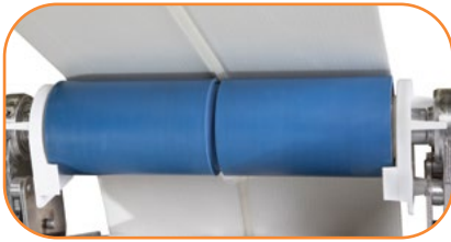
STANDARD FEATURE: V-Guided Belt Tracking
