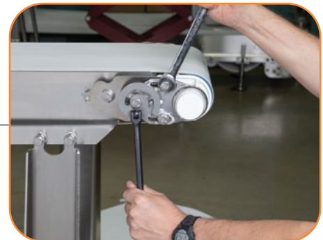
CAST ON URETHANE LAGGED PULLEY ENSURES A PERMANENT SANITARY BOND
