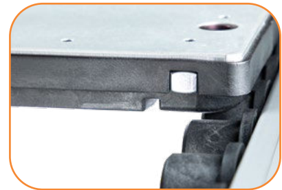
STANDARD FEATURE: Conveyor roller provides pallet guiding
