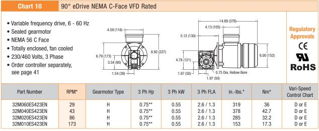
\* = At 60 Hz \*\* = Motor is de-rated to 0.5 Hp (2.2 / 1.1 amp) for full torque throughout the speed range.
