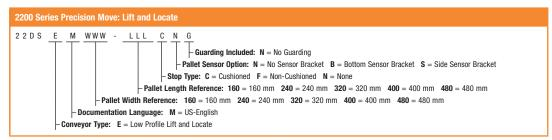
All combinations are valid except 160 mm width or length is not compatible with the bottom sensor bracket.
