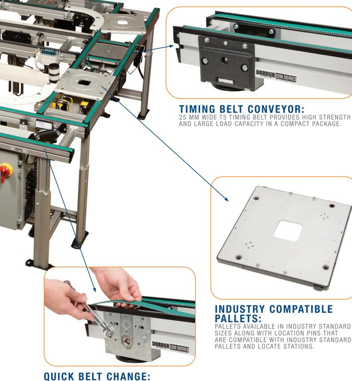
TOP REMOVAL BELT CHANGE METHOD PROVIDES QUICK BELT MAINTENANCE ACCESS WITHOUT THE NEED TO REMOVE THE CONVEYOR OR SURROUNDING AUTOMATION COMPONENTS.
