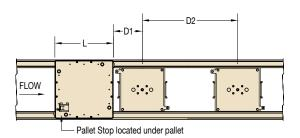
Pallet Stop to Lift & Transfer **Pallet Length** Minimum Minimum Minimum **Distance D2 Hardstop Distance D2 Cushion** L (mm) **Distance D1** 160 3.23" (82 mm) 10.35" (263 mm) 12.91" (328 mm) 13.50" (343 mm) 16.06" (408 mm) 240 4.80" (122 mm) 320 6.38" (162 mm) 16.65" (423 mm) 19.21" (488 mm) 400 7.95" (202 mm) 19.80" (503 mm) 22.36" (568 mm) 480 9.53" (242 mm) 22.95" (583 mm) 25.51" (648 mm)
