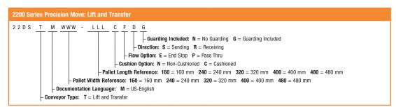
All combinations are valid except 160 mm width or length is not compatible with the bottom sensor bracket.
