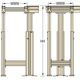
\*When motor is mounted vertical (position 4) stand minimum height 16".
