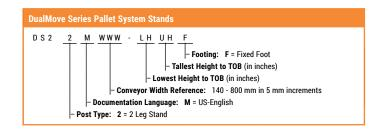
Note: Due to the wide variety of conveyor and stand options along with possible configurations, stability of the final setup is the responsibility of the end user. Note: Due to the wide variety of drive setups and applications, point of installation guarding is the responsibility of the end user. Note: Dimensions = mm (in)
