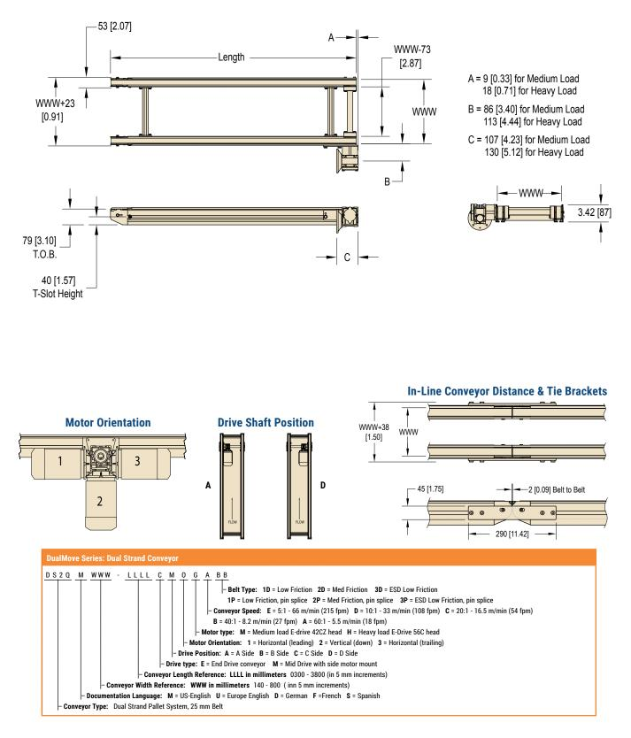
Note: Due to the wide variety of drive setups and applications, point of installation guarding is the responsibility of the end user. Note: Dimensions = mm (in)
