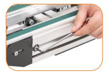
STANDARD FEATURE: Tensioning Mechanism
