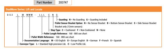
All combinations are valid except 160 mm width or length is not compatible with the bottom sensor bracket.
