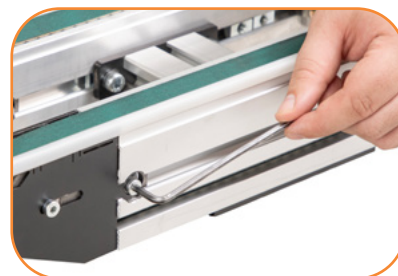
STANDARD FEATURE: Tensioning Mechanism
