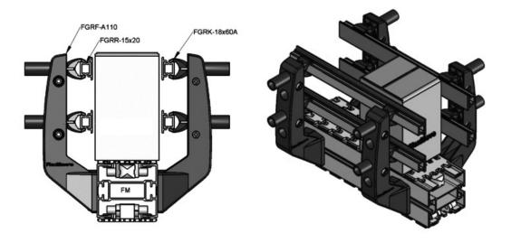
Width Adjustment Guide Rail Assembly
