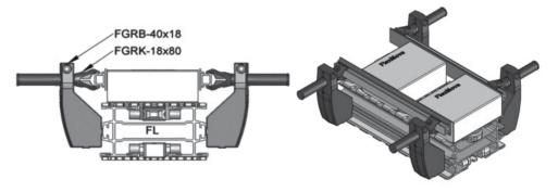
Width & Height Adjustable Guide Rail Assembly
