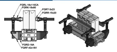
Width & Height Adjustable Guide Rail Assembly
