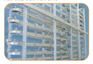
The Alpine Conveyor is a compact spiral configuration commonly used as an accumulation or buffer zone in between machines or as a process step for cooling or drying. It is also used for line balancing and for repair and maintenance purposes.
