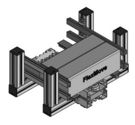
Width Adjustment Guide Rail Assembly
