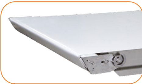
NOSE BAR TRANSFER OPTION FOR SMALL PRODUCT TRANSFERS. AVAILABLE IN: 12.7 MM (0.5 IN), 32 MM (1.25 IN) AND 48 MM (1.88 IN)
