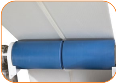
V-GUIDED BELTING FOR POSITIVE BELT TRACKING
